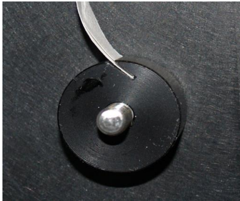
Figure 3-14: Insertion of Tape End into Take-up Reel
