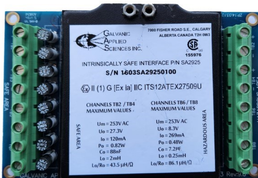
Figure 2-7: Intrinsically safe barrier SA2925.
