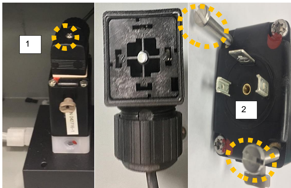
Figure 212: Installed Valve (Left); Valve Connector (Centre); Removing valve screws (Right)
