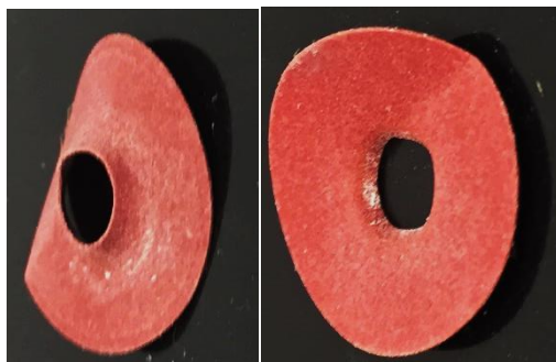
Figure 196: Deformed Piston Pump Seals
