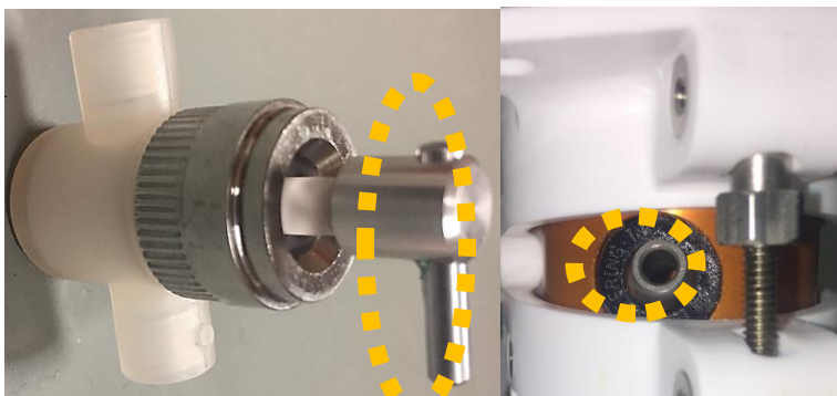
Figure 200: Piston with drive pin (left): Pump Assembly with Drive Bearing (right)
