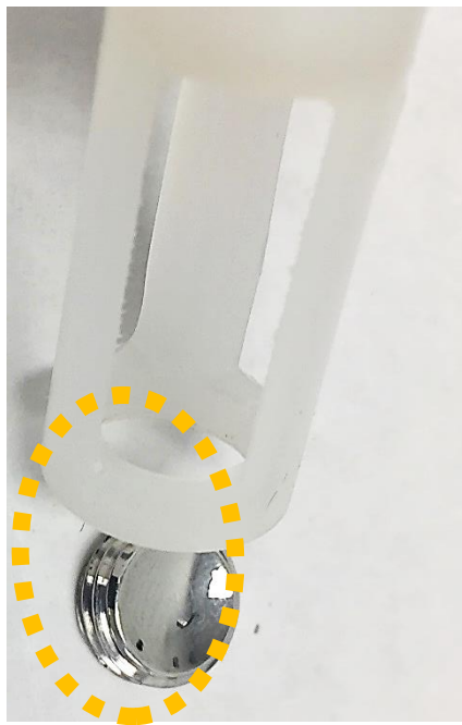
Figure 207: Optical Probe Tip w/ reflector removed
