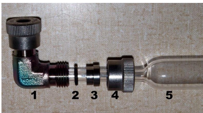
Figure 3-23: Exploded View of Ultra-torr Fitting
