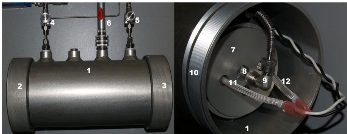
Figure 3-21: Total Sulfur Furnace Enclosure - Exterior (L) and Interior (R)
