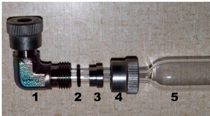
Figure7-6: Exploded View of Ultra-torr Fitting
