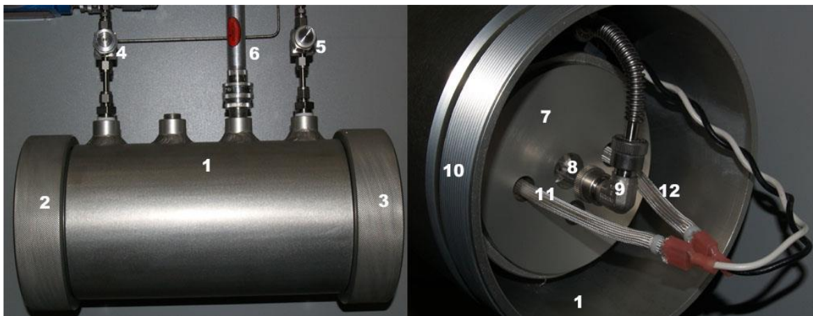
Figure 7-5: Total Sulfur Furnace Enclosure - Exterior (L) and Interior (R)
