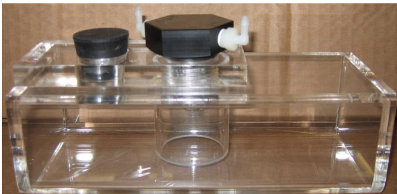
Figure 2-11: Total Sulfur Option Humidifier. Actual installed part may not be exact. Refer to Section 11 for individual part numbers.
