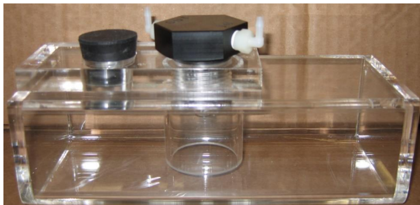
Figure 3-20: Total Sulfur Option Humidifier
