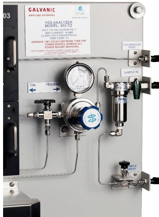
Figure 2-15: Typical Sample Conditioning System
