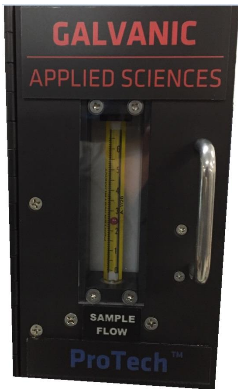
Figure 2-12: ProTech903 Chassis Rotameter without adjustment knob
