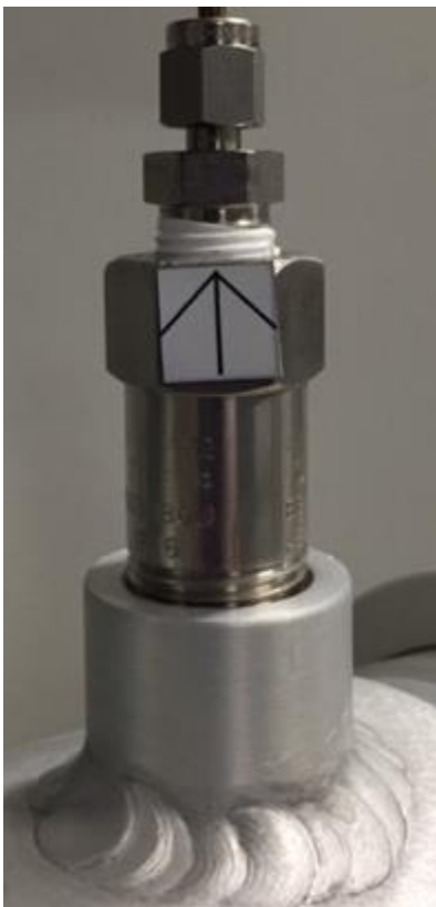
Figure 3-25: Location of Cap for Furnace Leak Check
