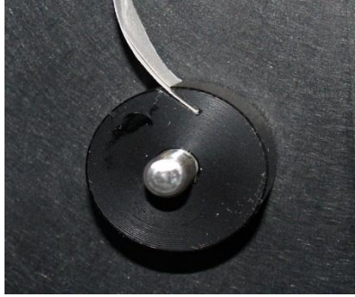
Figure 7-3: Insertion of Tape End into Take-up Reel
