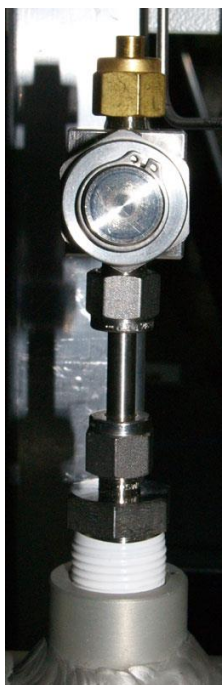
Figure 7-7: Location of Cap for Furnace Leak Check
