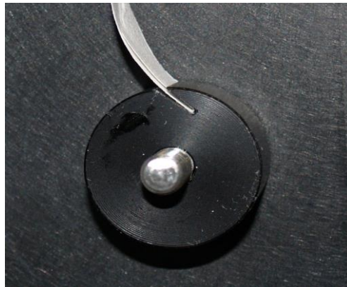
Figure 3-14: Insertion of Tape End into Take-up Reel
