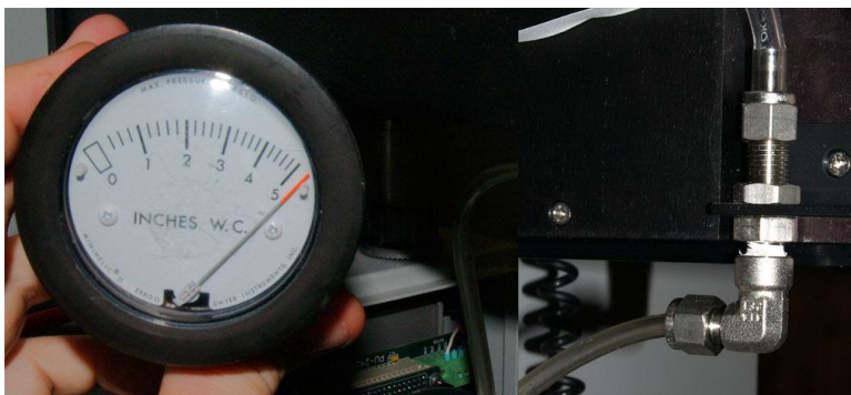
Figure 3-21: Minihelic Indicating a Good Seal (L); Connected to Vent Elbow (R)
