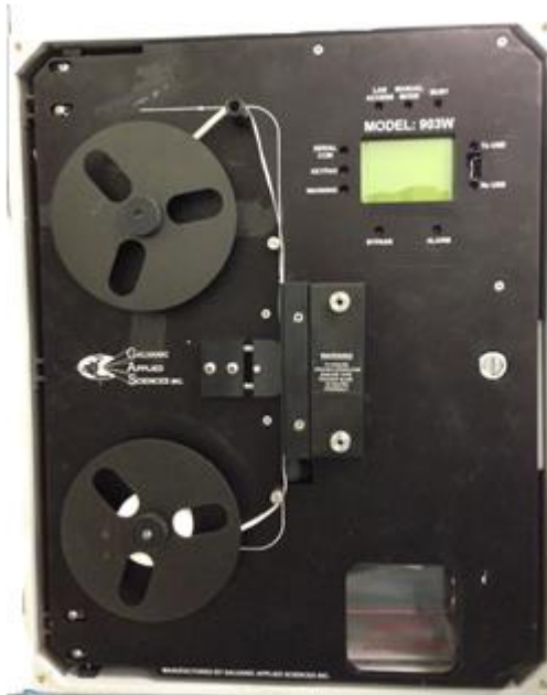
Figure 2-3: Tape Transport System
