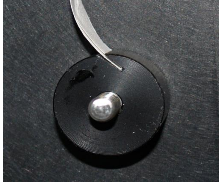
Figure 7-3: Insertion of Tape End into Take-up Reel
