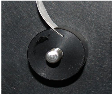
Figure 7-3: Insertion of Tape End into Take-up Reel
