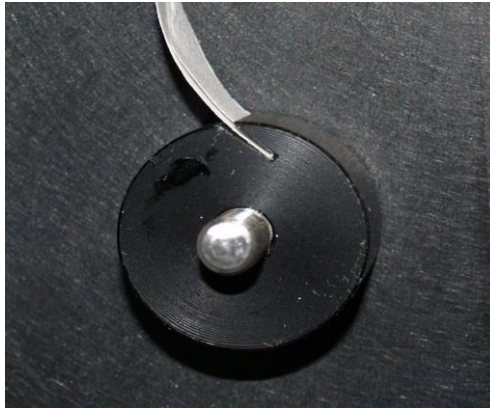
Figure 3-16: Insertion of Tape End into Take-up Reel
