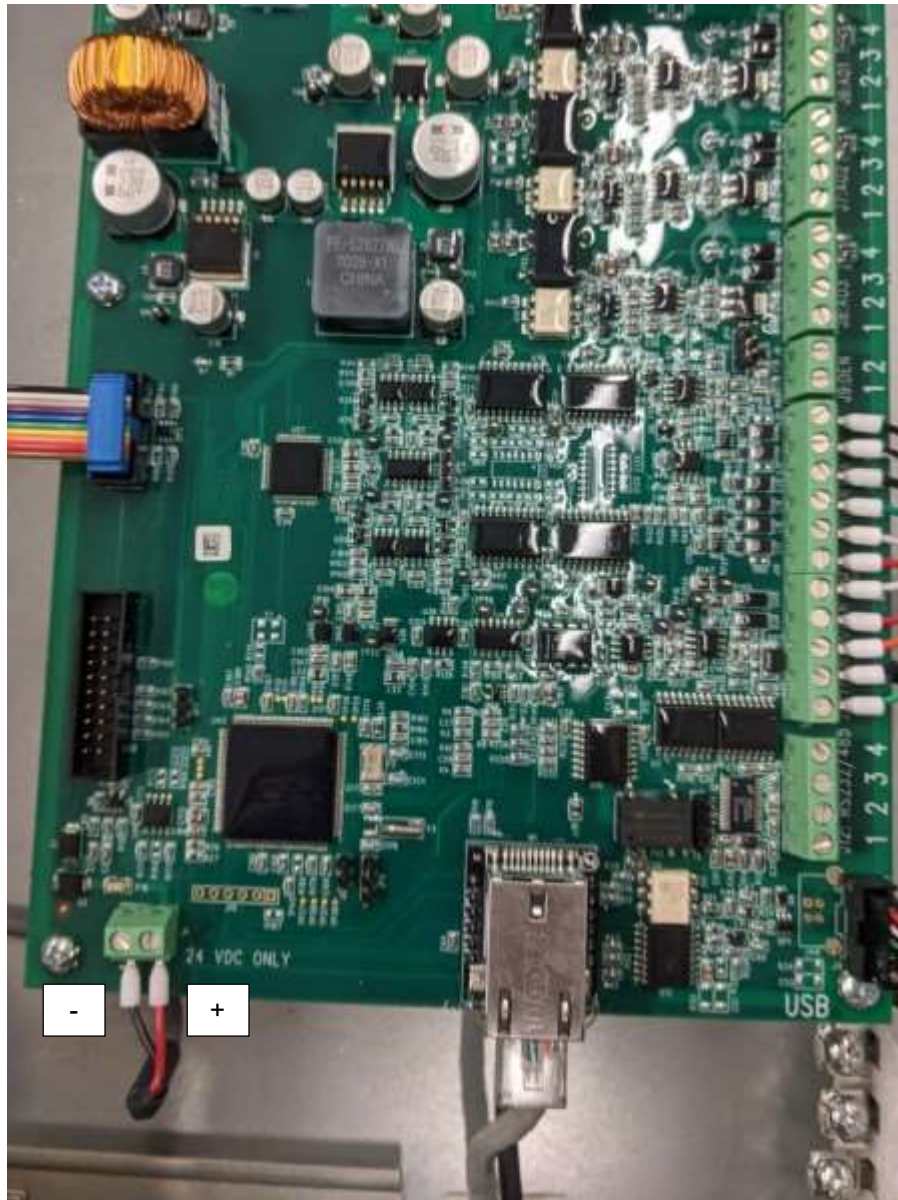
Figure 5: Power Connection for DC Powered Viscometer
