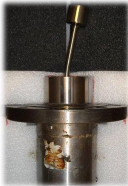
Figure 6.3: Bent (Damaged) Transducer
